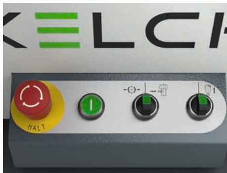
Control panel for spindle functions
