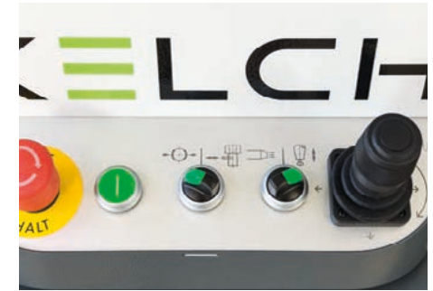
Control panel with joystick to move the CNC axes.
