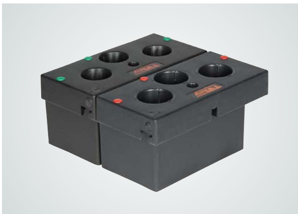
TUL mounting plates · Basic element of the TUL system · Available in different designs (for example refer to the TUL range for holding tools, inserts for modular precision spindles or other tools) · Required space: L x W x H = 240 x 120 x 130 mm
